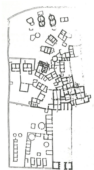
Figure 3.22: Layout of the Palace of Emir of Zaria showing the zaure, cikin gida, kofa gida, sleeping quarters, shigifa and rest of the Palace compound Source: Dmochowski, 1990 Vol. I.
