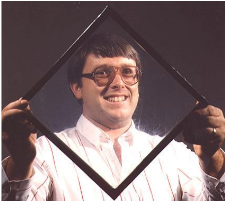
Fig. 8: Prototype of double paned glazing unit filled with aerogel at Lawrence Berkeley National Laboratory.
